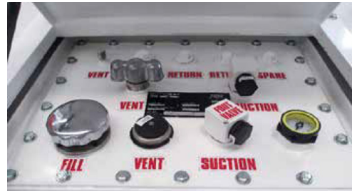
Typical Inner Tank Configuration
