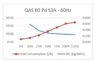
(Reference conditions at 25°C Air Inlet Temperature, 60% Relative Humidity, 1bar Absolute inlet pressure, for different conditions or limitations contact Atlas Copco technical support).
