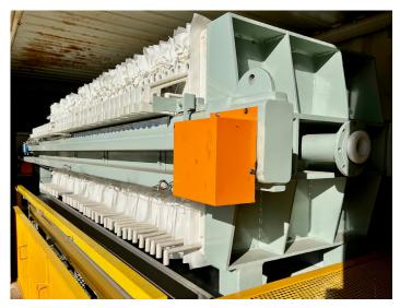
The sludge press is a key component of NPE's waste water and by-product management systems. The majority of NPE's water treatment methods produce liquid waste as they remove contaminants from effluent and store them temporarily in a more concentrated form (sludge). Although these volumes are small relative to the volumes of clean water produced, they are tricky to manage on small sites and are expensive to dispose of over the course of a project.
