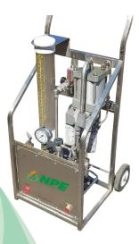
The air-driven high-pressure pumps used in the chemical injection unit are particularly built for maximum performance and efficiency. The device has been developed for both on and offshore operations and is housed in 316 Stainless Steel trolley for portability.
