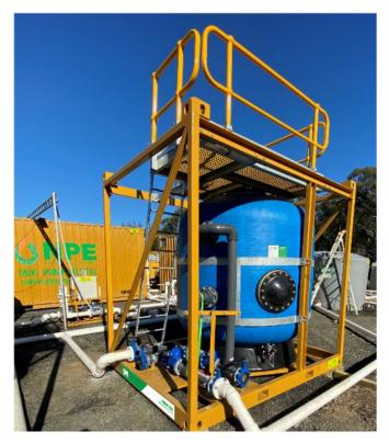
The Multi Media Filtration Unit (MMFU) offers a flexible and effective solution for various water treatment requirements. The MMFU is suitable for a variety of filter medias and treatment requirements including but not limited to sand/glass filtration, ion exchange, activated carbon, catalytic media, and a variety of other filtration medias on the market.
